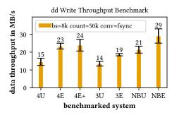
Figure 2: Results of the dd microbenchmarks. In the legend, the 3 and 4 indicate the respective Pi, NB indicates the Notebook, U, E, and E+ indicate the Ultra and Evo(+) MicroSDs. For example, 4E+ refers to the Evo+ card in a Pi 4.
